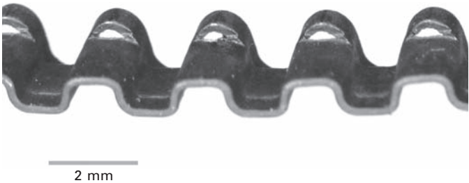
4.1 (a) Piston rings for a four-stroke engine. Top and second rings (two rings on the left) and assembled three-piece oil control ring (on the right). (b) Disassembled three-piece oil ring. (c) Magnified view of the spacer. There is also a one-piece oil ring.
