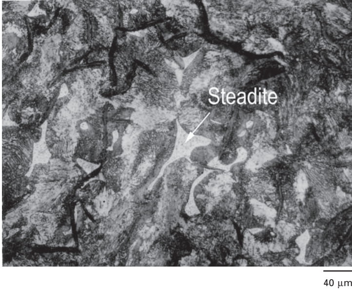
2.16 High-P cast iron. The matrix has a pearlite microstructure, being a mixture of cementite and ferrite. Steadite is a eutectic crystal containing \text{Fe}_3\text{P} compound and ferrite. It appears typically in the cast iron of 0.3% P and over. See Appendix D.
