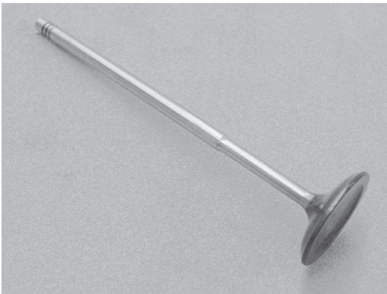
6.1 Exhaust valve. The inlet valve has a similar shape, but the crown size is normally larger than that of the exhaust valve.
