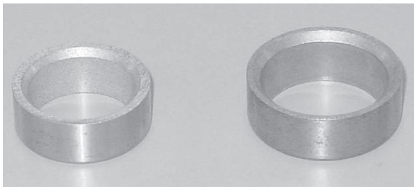
6.17 Valve seat inserts for inlet (right) and exhaust (left).
