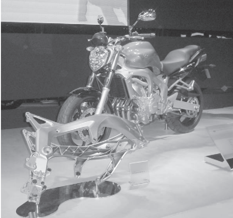
J.3 Thin-walled frame made by high-pressure vacuum die casting. The motorcycle with the frame installed is also shown on the right.
