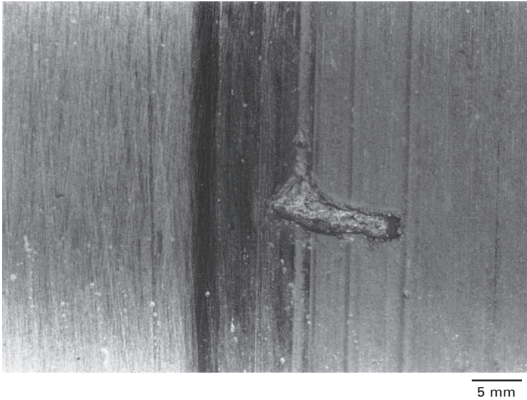
8.13 Pitting observed at a crankpin surface.
