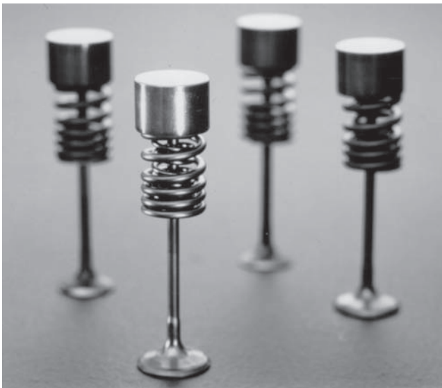
7.2 Double springs installed in a bucket type valve lifter.
