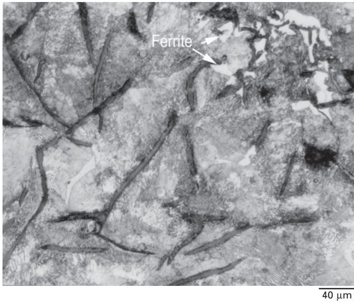
2.7 Microstructure of a gray cast iron (JIS-FC200) block.
