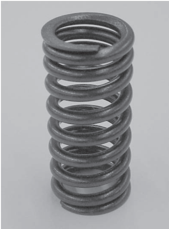
7.1 Valve spring. Generally, coil springs of a wire diameter below 5 mm \phi are cold-formed at room temperature, while wires above 11 mm are normally hot-formed. Compression valve springs are provided with the ends plain and ground.
