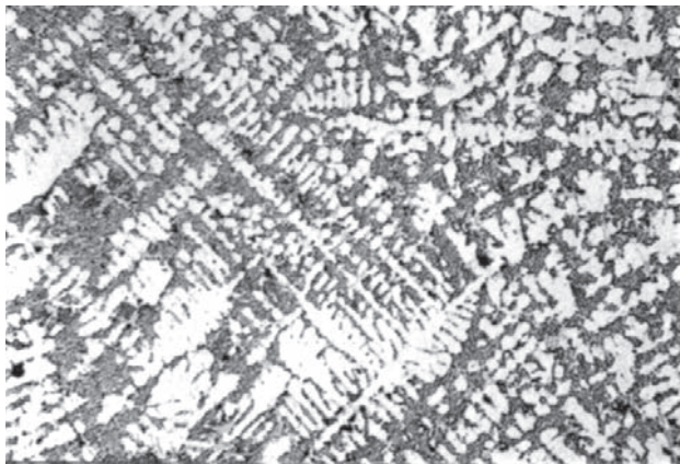
3.12 Dendrite crystals of AC8A. White portions are crystals having a composition close to pure aluminum. Surrounding gray portions containing a higher Si concentration solidified at a later stage.
