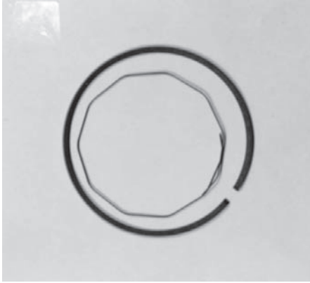
4.4 Piston rings for a two-stroke engine. The expander put at the center takes free state. When set into the piston ring groove, it spreads and gives additional force from the back of the second ring as shown in Fig. 4.9.
