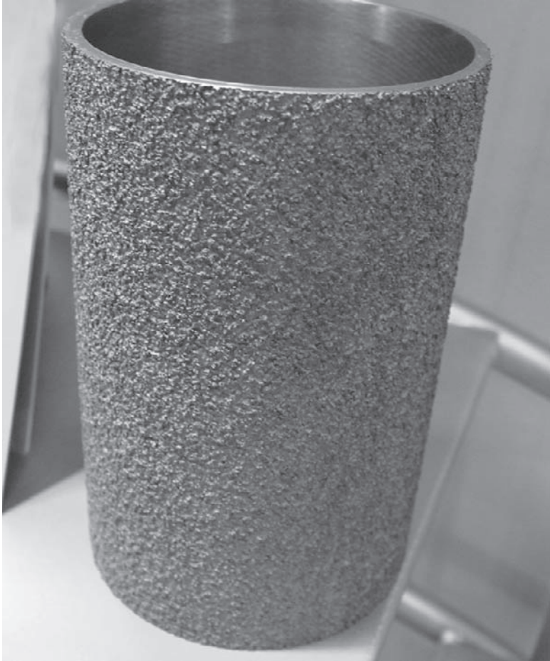
2.20 Cast iron liner having dimpled outer surface.
